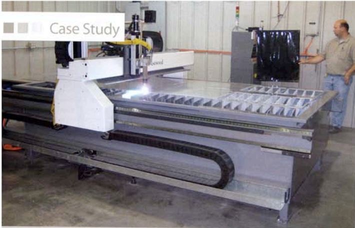
◀ Kyle Ashleman programs ButlerBuilt's plasma table to cut aluminum parts.
