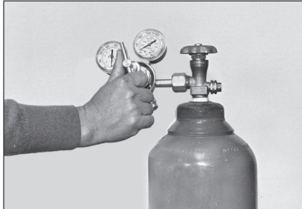
5. Both cylinder valves and regulator connections should be checked for leaks. Stand so the cylinder valve is between you and the regulator. **SLOWLY OPEN THE CYLINDER VALVE** to avoid Diaphragm damage in regulator. An approved leak detector should be used.
