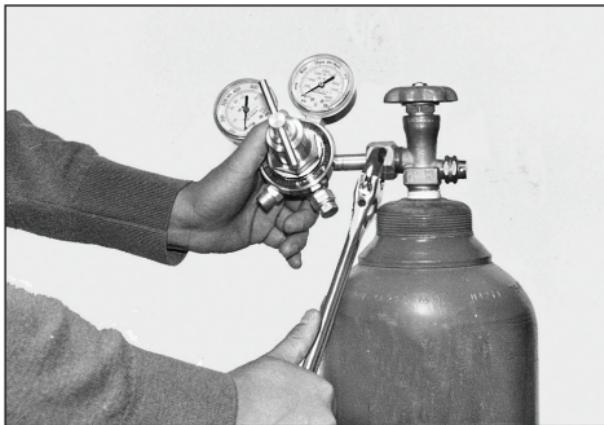
4. Regulator adjusting screws should be turned counterclockwise to relieve pressure on diaphragm before opening cylinder valves. If this is not done, pressure from cylinder can damage diaphragm and render regulator inoperable. See Picture on the next page.
