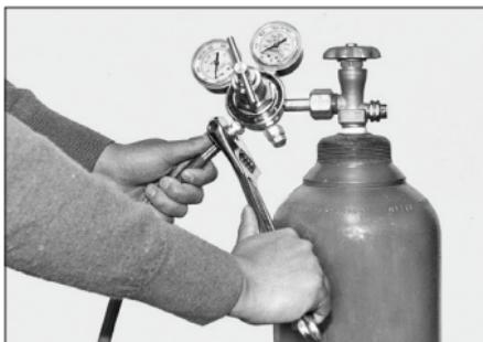
7. Purge the new Hoses: Before using a brand new welding hose which contains a preservative talc, clear the residue in the hoses in a well-ventilated area and away from flammable substances with the following procedures:
