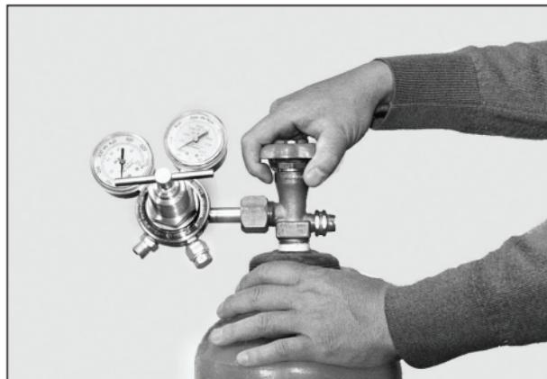
6. Connect proper hose to regulator. (Green to oxygen and red to acetylene.) Tighten nuts securely with wrench.
