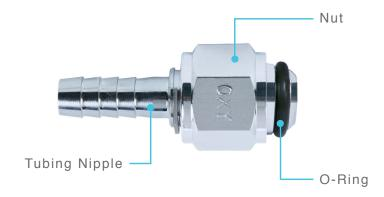
The nut and tubing nipple are made of nickel-plated brass. The adapters are meant for multiple uses, not single patient use. If you would like to sterilize the nut and tubing nipple, please remove the O-ring from the tubing nipple. The reusable nut and tubing nipple are primarily used with oxygen & air flowmeters, and can be wiped down. They can also be cleaned with soap detergent & water as well as PDI wipes, BPI wipes, Hypo-chloride wipes and Quaternary wipes.
