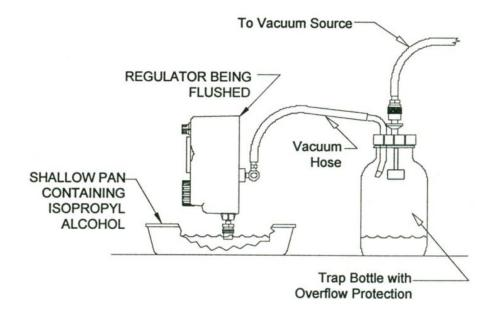
• Turn the mode selector switch to OFF. Attach two vacuum hoses as shown below. The collection bottle will trap the liquid and keep it out of the hospital vacuum system. Place the patient conection of the GENTEC<sup>®</sup> regulator into a shallow pan containing isopropyl alcohol.
