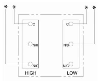
\* Terminals to be used for Genstar Technologies alarm panels and other systems sensing fault on electrical contacts opening.
