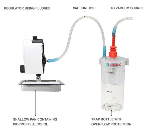
1 Turn the mode selector switch to OFF. Attach two vacuum hoses as shown above. The collection bottle will trap the liquid and keep it out of the hospital vacuum system. Place the patient connection of the GENTEC<sup>®</sup> regulator into a shallow pan containing isopropyl alcohol.
