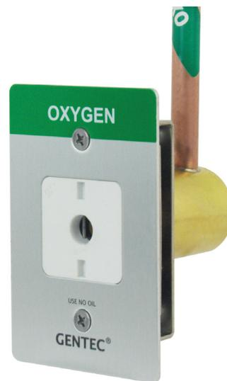
Universal rough-in assembly shall include a rough-in plate (16 ga.) with gas inlet tubing silver brazed to the outlet body. Inlet tubing shall be type "K" copper, 1/2" O.D. (12.7 mm), extend 6-1/2 inches (165 mm), and swivel 360° for ease of installation. Rough-in assembly shall accept only the specified gas service by use of indexes. A dust plug shall be provided to protect rough-in assembly from contamination during and handling and installation.
