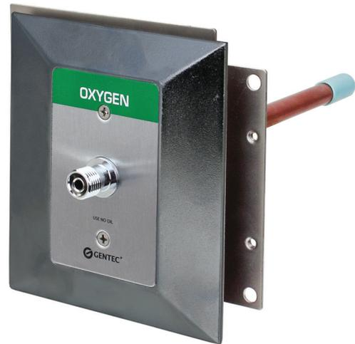
Universal rough-in assembly shall include a rough-in plate (16 ga.) with gas inlet tubing silver brazed at 180 degrees to the outlet body. Inlet tubing shall be type “K” copper, 1/2” O.D. (12.7 mm), and extend 6-1/2 inches (165 mm).
